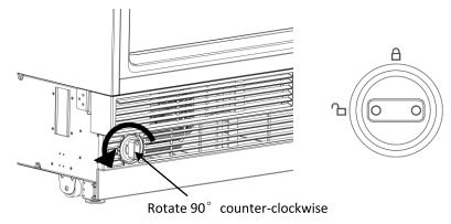
Insert the water filter – with the knobs at the front in a horizontal position As far as it will go, and turn clockwise until it snaps in.
